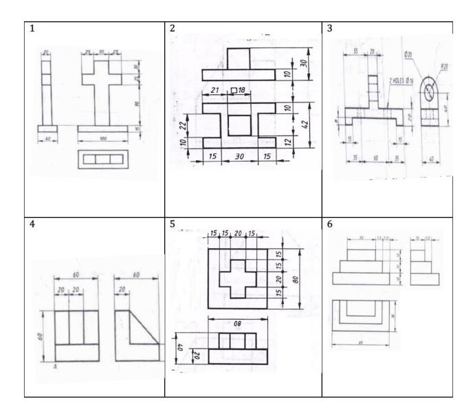
3. Draw the isometric Projection of the machine component whose orthographic views are given
