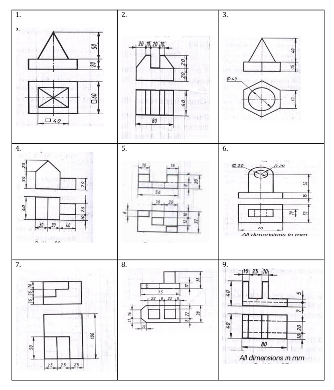
2. Draw the isometric Projection of the machine component whose orthographic views are given below:
