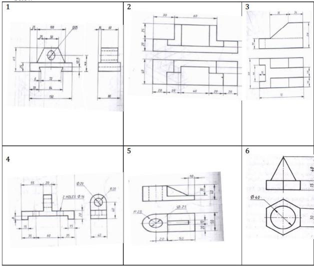
4. Draw the isometric View of the machine component whose orthographic views are given below
