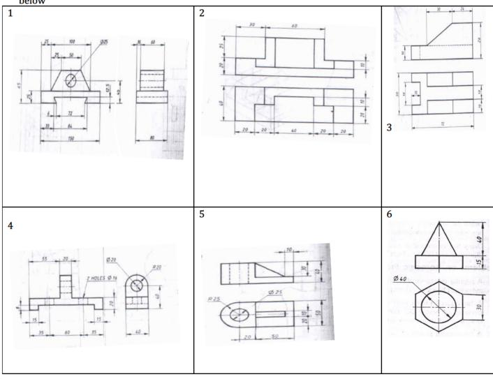
3. Draw the isometric Projection of the machine component whose orthographic views are given below
