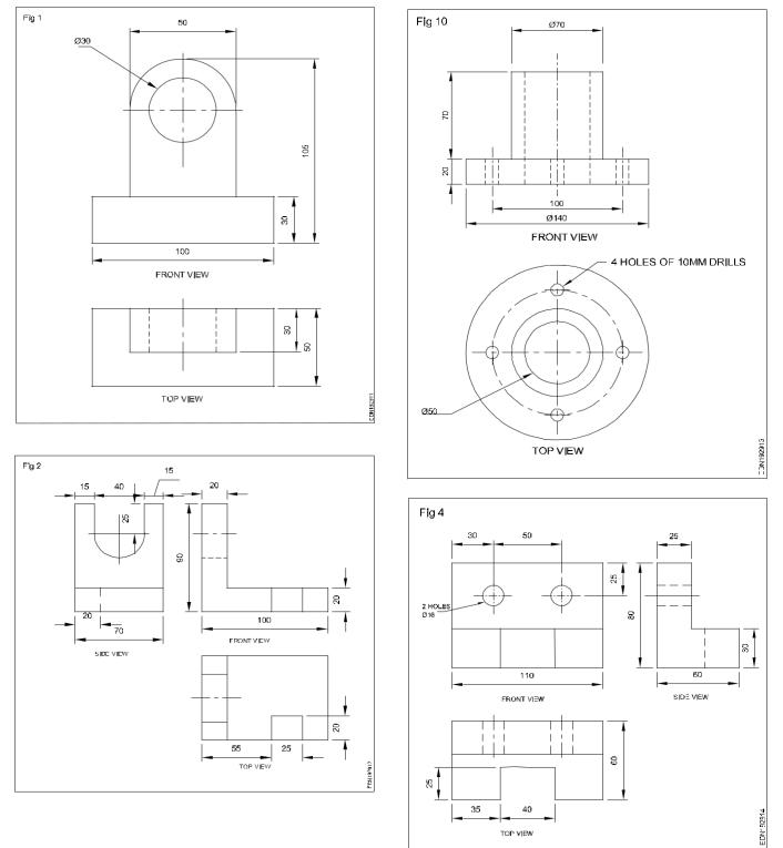
4. Draw the isometric View of the machine component whose orthographic views are given below
