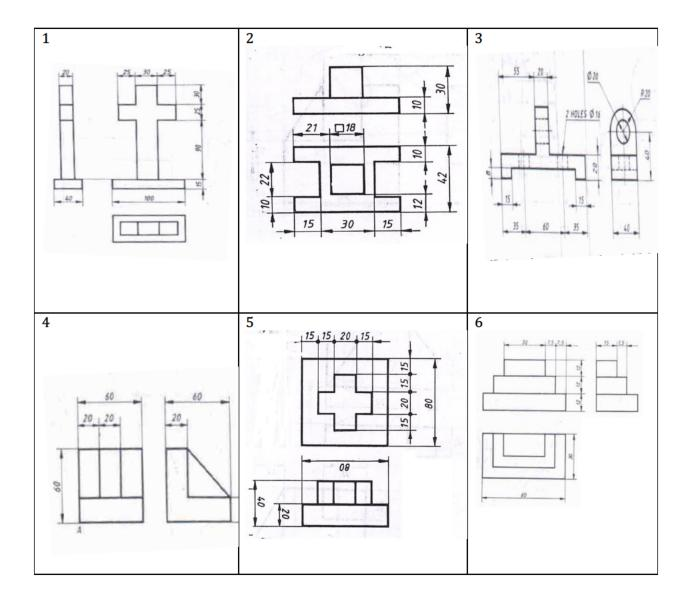
2. Draw the isometric Projection of the machine component whose orthographic views are given below:
